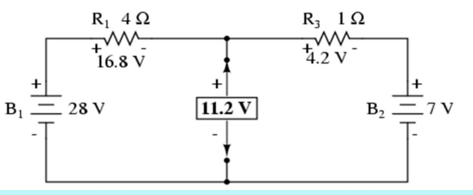
$V_{\text{Theveni'n}}$  is the open circuit voltage from where load is removed
