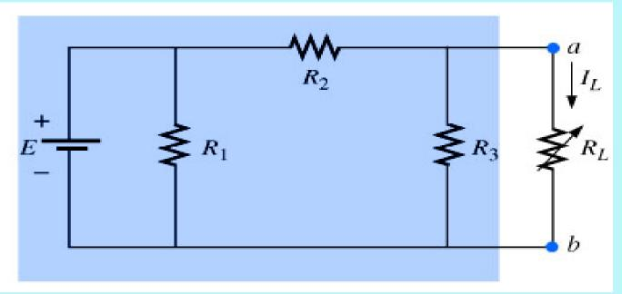
2. Mark the terminals of the remaining two-terminal network. (The importance of this step will become obvious as we progress through some complex networks.)
